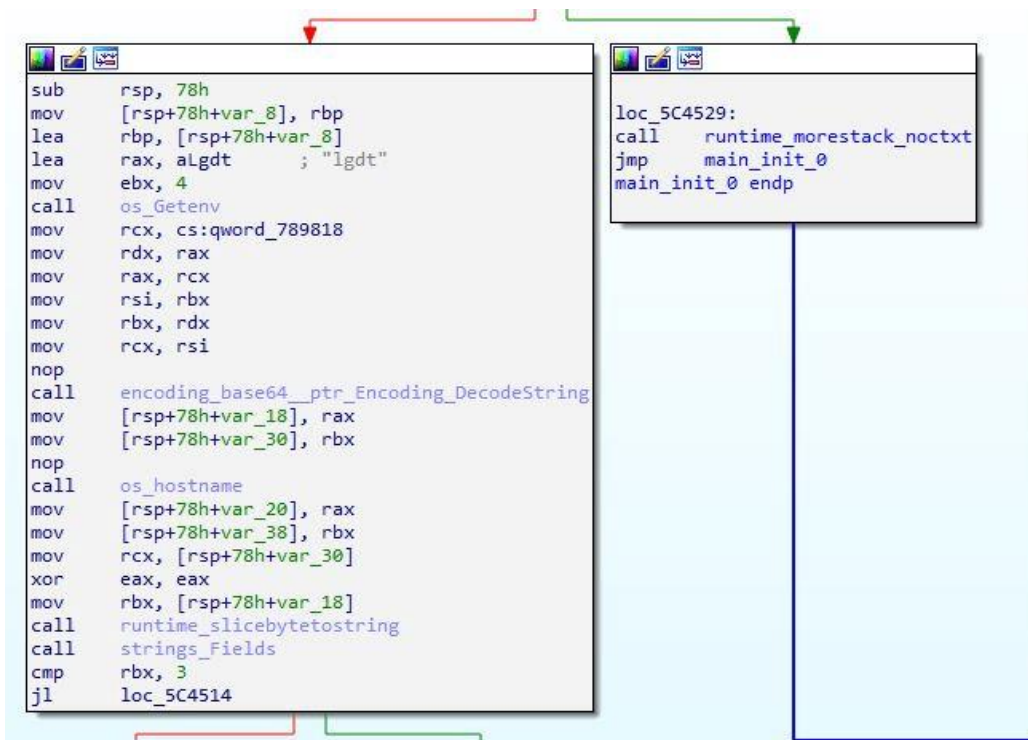
Figure 10. Routine that decrypts environment variables and uses them as configuration data
