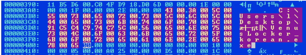
Figure 2. Strings within the LNK file that signify the creator is the same
